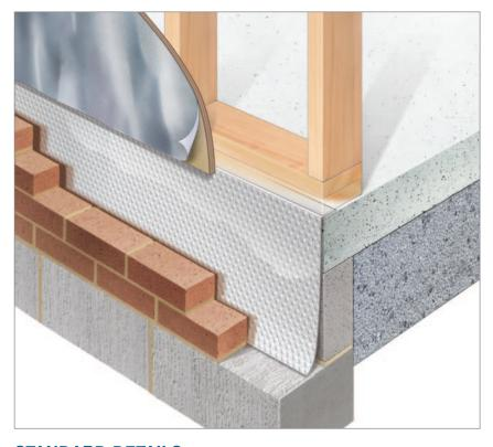
A simple and low cost solution for insulating the edges of ground floor slabs to prevent cold bridging.
