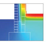
Assessing thermal bridges and calculating their linear thermal transmittance (PSi value or Ψ value) and temperature factor to evaluate the risk of surface condensation and mould growth.
