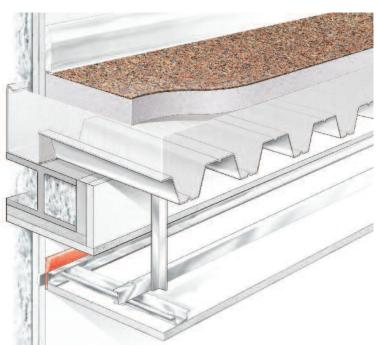
Our innovative and durable acoustic products are designed to minimise the transfer of airborne and impact sound. Products are designed for under screed, soft coverings, floating floors, structural deck and vibration isolation application. These include the Isorubber, Dekfloor and Isovibra ranges.
